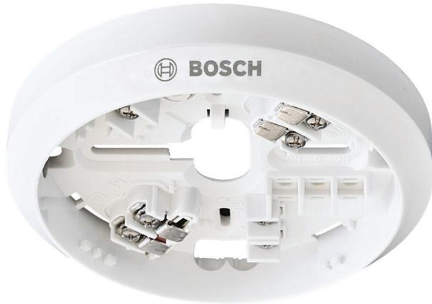
The MS 420 can be used to mount detectors from the 420 Series, and has integrated jumper elements that preserve the loop function if the detector is removed. To protect against unauthorized removal, the detector head can be secured with a variable locking.
